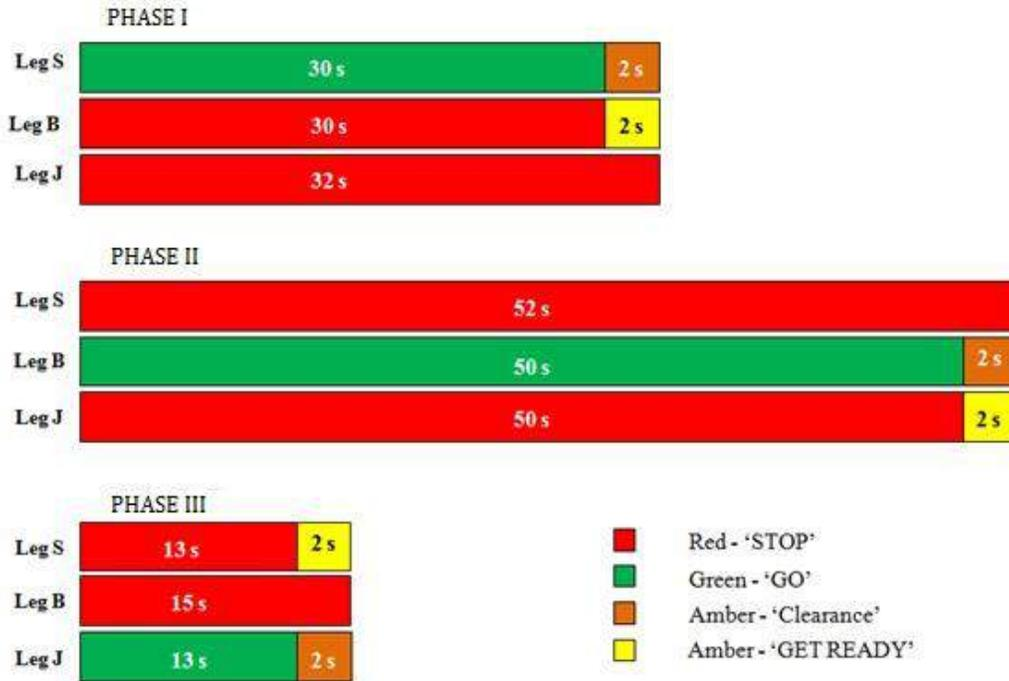
Fig.10.1 Illustration showing 3-phase signal timing diagram
