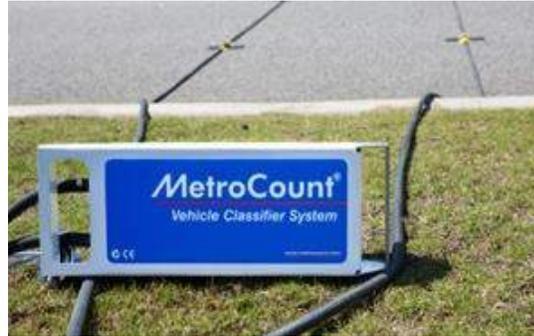
Fig 2.4 Pneumatic tubes installed on road connected with the sensor
