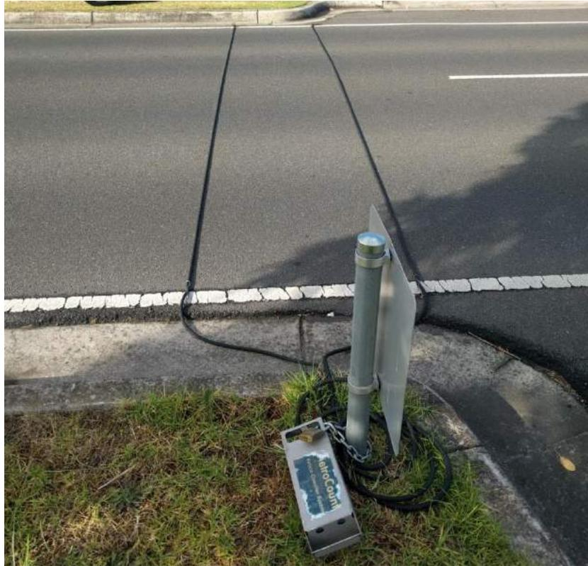
Fig 2.5 Pneumatic tube installed on a road
